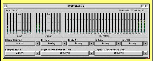
The first four (or eight) meters show the input levels, and the next four (or eight) show the output levels.
