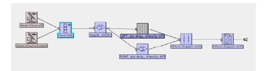
The upper half of the Sound editor shows you the signal flow of the modules that make up the Sound. This is also where you can modify the Sound by adding or deleting modules from the signal flow diagram.
