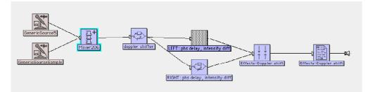
If you were to drag <u>Effects-Doppler shift</u> and drop it onto a Sound in the timeline, the replaceable input is the module within it that will be replaced by the Sound in the timeline.
