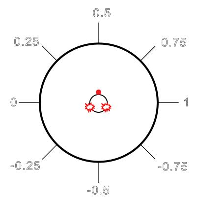
A sound source directly to Bozo's left is at angle 0, a sound source directly in front of Bozo is at angle 0.5, and a sound source to your right is at angle 1. (If you multiply these numbers by 180 degrees (or by pi), they will correspond to familiar angles). Positions *behind* you are the negative versions of the ones in front of you.
