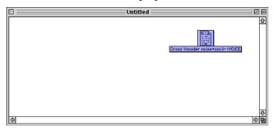
What if you want to drag a Sound from the browser into a Sound file window with its *original* input (rather than the replacement input)? To do so, disconnect the replacement input first (by clicking on the button with the yellow arrow just to the right of the replacement input field); *then* drag the Sound into the Sound file window.
